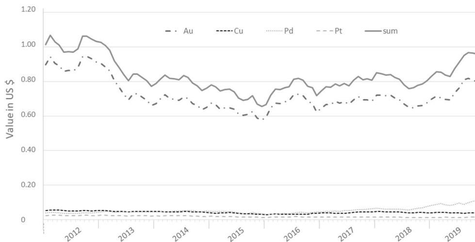
Fig. 3. The value of Au, Pd, Pt, and Cu based on their fractional content in smartphones, calculated over the timeframe 2012–2019. The top line represents the sum of their fractional values.
